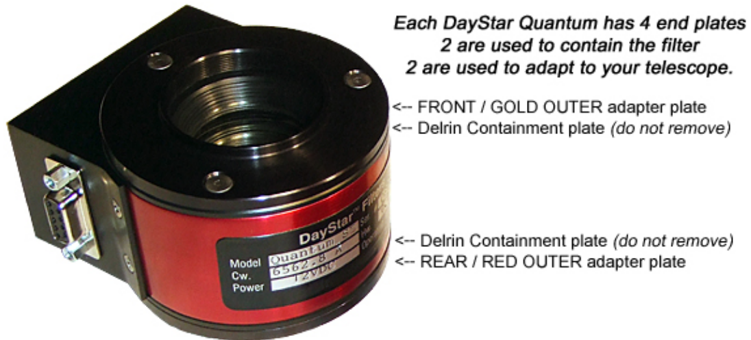
Figure 25: Quantum adapter plates (see next chapter for available options).
