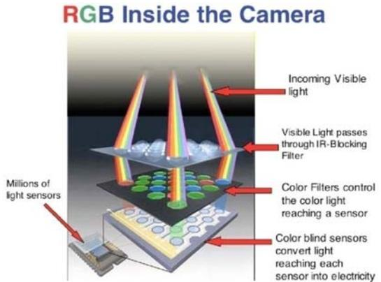
The DSLR imager must be aware that most camera manufacturers (Canon and Nikon) use an IR blocking filter which greatly reduces the transmission of Hydrogen Alpha light. DSLR cameras without this IR blocking filter will have better sensitivity imaging in Hydrogen Alpha.
