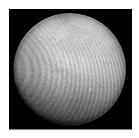
Another effect present in CCD imaging of monochrome light of Magnesium is the interference pattern - or Newton's Rings. The effect is similar to interference testing of an optical surface between two flat surfaces. The sensor and cover slip cause a small interferometer inside the camera and cause a Newton's Ring moire' pattern. The CCD chip must be tilted to a minor degree to prevent this pattern. Recent advances
